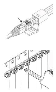
The One-Click® Cleaner MPO is an easy-to-use option for cleaning MPO and MTP® multi-fiber connectors used in data centers and other high density optical networks. One-Click Cleaner MPO is a revolutionary push-type cleaner, which simplifies cleaning of the ferrule end-face of both MPO/MTP exposed connectors and connectors in adapters.
