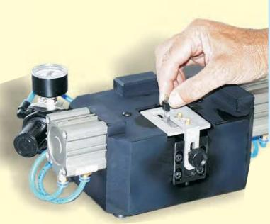
A pneumatic machine designed to cut loose radial component leads.
