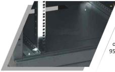
New profile fixing system efficiently increases maximum load capacity of the cabinets and facilitates cable management. Profile rails with 25 mm hole spacing arranged horizontally at the top and the bottom of the cabinet, for fixing and depth adjustment of the mounting rails. Minimum distance from the front door and front profile rails - 95 mm.
