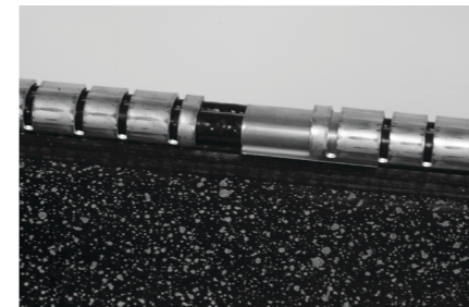
15 Slide the flexible channels over the sleeve rails leaving a small gap at the center for the underclip. Position the underclip in the opening between the channels and slide the channels evenly over the clip.
