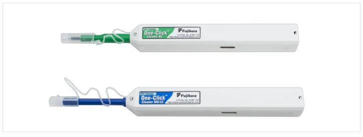
The Fujikura One-Click™ cleaners are mechanical cleaning tools designed to clean connectors residing in an adaptor or faceplate and unmated connectors. The Fujikura One-Click™ cleaners use a novel dry cleaning strand to gently sweep and lift away dust and residues from the connector end face.
