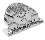
FIST® Splice Sub-assembly kit with 4 trays, each for holding up to 12 primary or 4 secondary coated fibers, with Heat Shrink type splice holder
