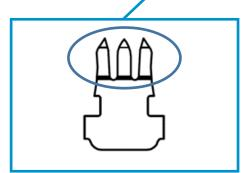
The triple pin blades provides higher electrical conductivity
